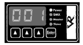
**Power light** (red). This light should be on whenever the unit is powered up. If it doesn't come on there is either no power to the unit, or some internal problem with the unit.
